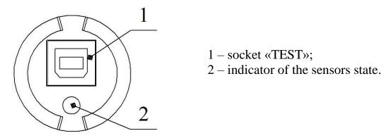
Figure 1.6 – Configuration elements of the Rx unit of the sensors BARRIER-24.M (general purpose)
