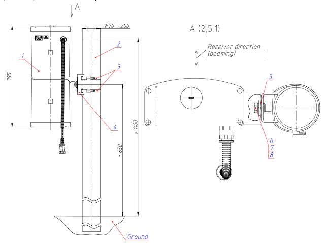
1 – Tx unit (Rx unit); 5 – plastic washer; 2 – pole; 6 – bolt M8; 7 – washer 8;
