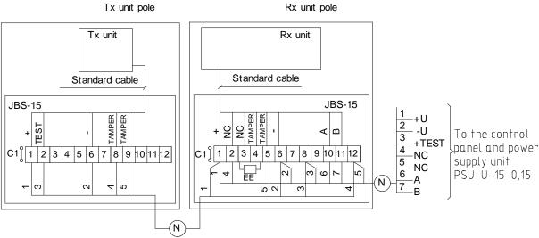
Figure 2.10 – Diagram of connection the sensor using the junction box JBS-15.
