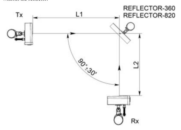
Figure 2.14 – Installation of the sensors using REFLECTOR-360 (REFLECTOR-820)
