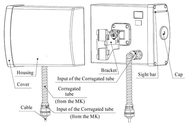
Figure 1.4 – The design of the Tx unit (Rx unit) of the sensors BARRIER-24.M50, BARRIER-24.M100, BARRIER-24.M200
