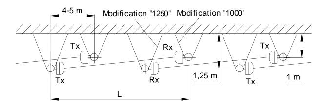
Figure 2.6 – Example of installation of the sensors BARRIER-24.M (general purpose) on BRACKET-1000, BRACKET-1250 with overlapping the detection zones
