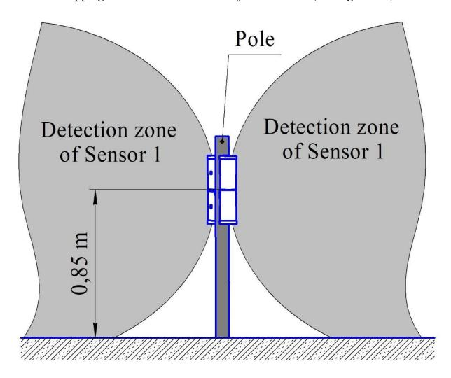
Figure 2.2 – Installation of Rx units (Tx units) of the sensors BARRIER-24.M300, BARRIER-24.M500 on one pole without overlapping the adjacent detection zones
