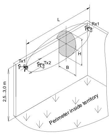
Figure 1.3 – The shape of the detection zone generated by the sensors BARRIER-24.M50, BARRIER-24.M100, BARRIER-24.M200 installed on the fence
