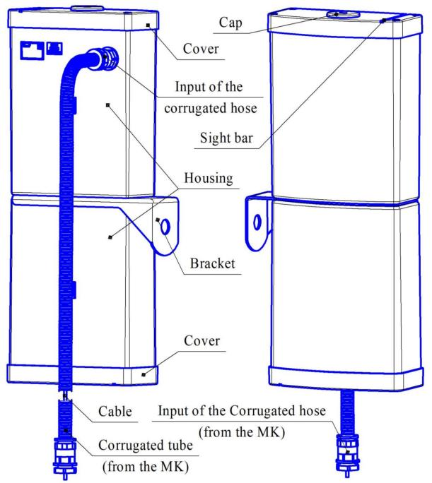
Figure 1.5 – The design of the Tx unit (Rx unit) of the sensors BARRIER-24.M300, BARRIER-24.M500
