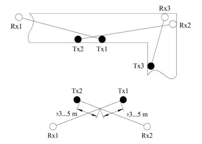
Figure 2.1 – Example of perimeter marking for sensors installation
