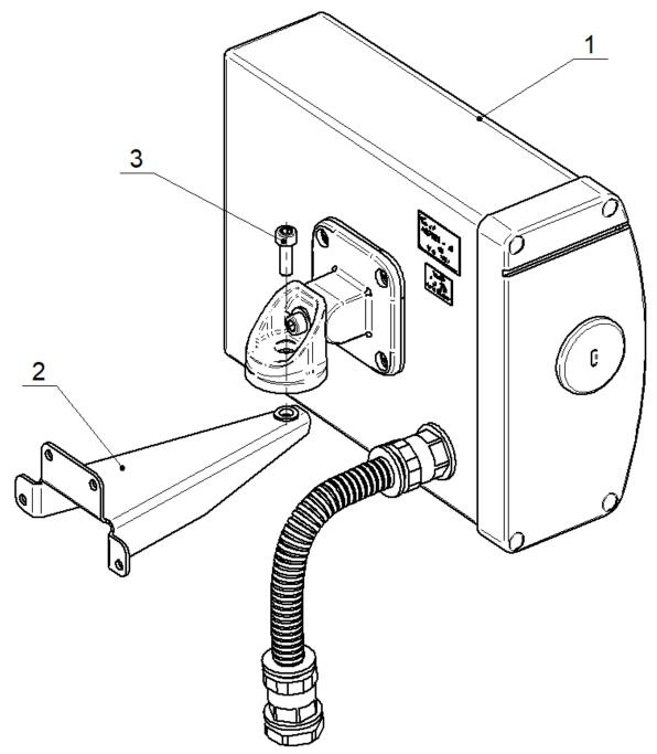
1 -Rx unit (Tx unit); 2 - BRACKET-120M; 3 - screw M5
